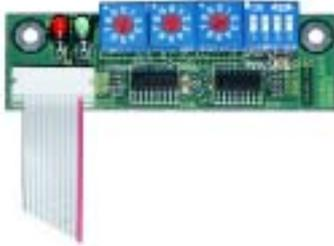
The start address setting board is used to set the number of the DMX start address, that is the number of the first data slot used by the 3032R relay card. The card then uses 32 consecutive data slots to switch the outputs accordingly. Setting of the switches is straightforward decimal.
